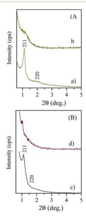
Fig. 2 Low-angle XRD patterns of mesoporous pristine carbon (A) and nitrogenous carbon (B): (a) CSI-809, (b) LFP/CSI-809, (c) MNC-859, and (d) LFP/MNC-859.
