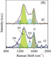
Fig. 4 Raman spectra of pristine OMC (A) and nitrogenous carbon (B): (a) CSI-809, (b) LFP/CSI-809, (c) MNC-859, and (d) LFP/MNC-859.
