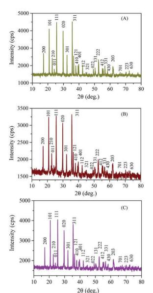
Fig. 1 Wide-angle XRD patterns of (A) LFP/CSI-809, (B) LFP/MNC-859, and (C) LFP.
