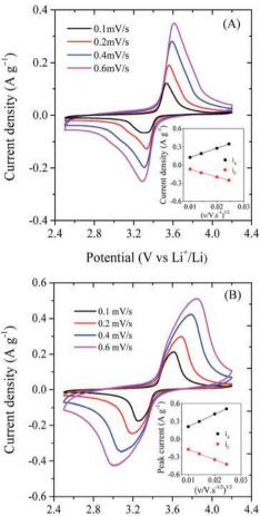
Fig. 6 Cyclic voltammograms of (A) LFP/CSI-809 and (B) LFP/MNC-859 at different scan rates. Insets: relationship between the peak currents and  $v^{1/2}$  at various scan rates.
