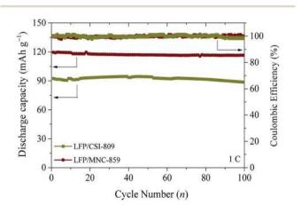
Fig. 9 Cycling stability studies of the LFP/CSI-809 and LFP/MNC-859 electrodes at the current rate of 1C.
