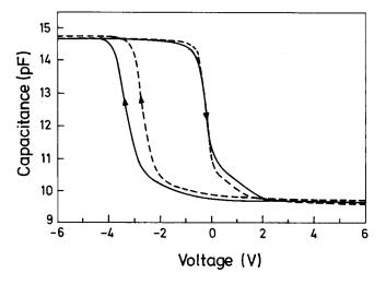
FIG. 1. C-V characteristics of freshly prepared Al-xerogel-pSi MIS device at 1 MHz (solid line) and after aging for 40 days (dashed line).
