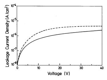
FIG. 2. Leakage current density–voltage characteristics of freshly prepared Al–xerogel–pSi MIS device (solid line) and after aging for 40 days (dashed 129.1 line).
