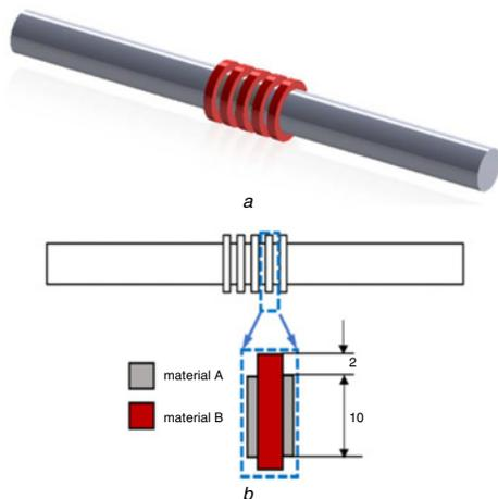
**Fig. 3** Design of the elastic metamaterial rod with baffles
