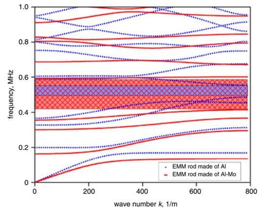
**Fig. 8** Comparison of dispersion curves achieved by using single and bimetallic EMM rod
