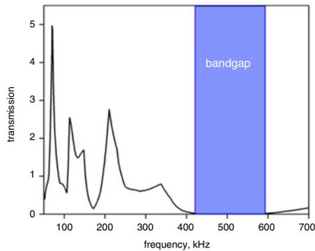
**Fig. 6** Transmission spectra of EMM rod with baffles computed along direction of wave propagation
