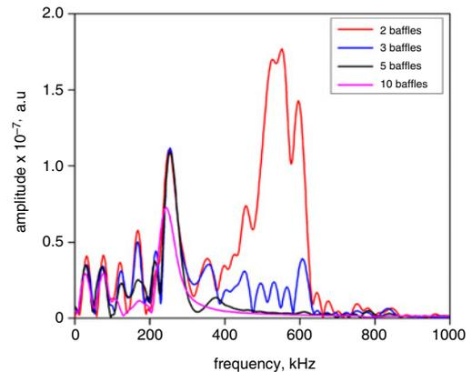
**Fig. 5** Effect of number of baffles on bandgap
