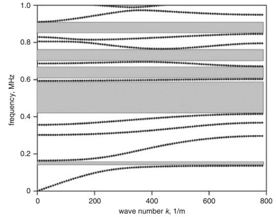
**Fig. 4** Band structure observed from EMM rod with baffles
