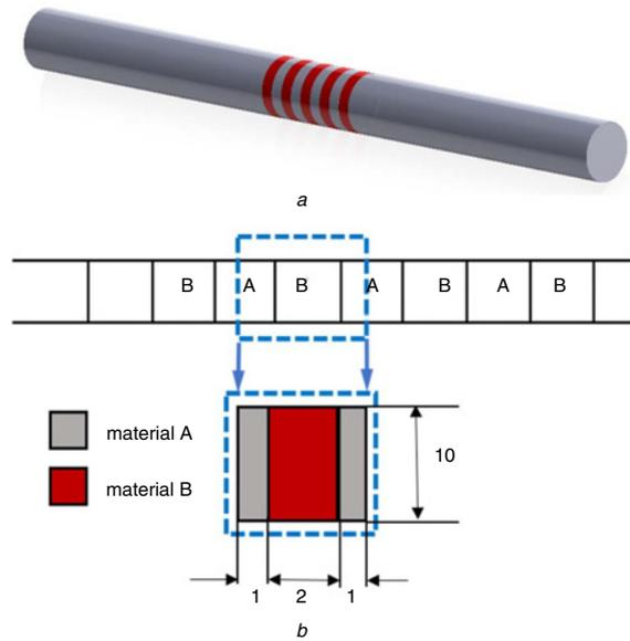
**Fig. 1** Illustration of the proposed bimetallic rod
