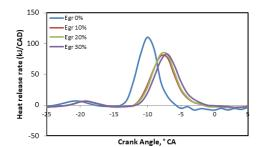
Fig. 17. Variations of HRRs with the EGR rate at the boost pressure of 1.1 bar.
