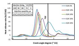
Fig. 13. Variations of HRRs with EGR rate with five pulses injection.
