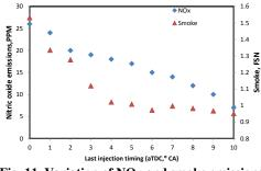
Fig. 11. Variation of NOx and smoke emissions with last injection pulse timing with five pulses Injection.
