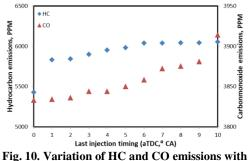
Fig. 10. Variation of HC and CO emissions with last injection pulse timing with five pulses injection.
