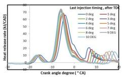
Fig. 9. Variations of HRRs with last injection pulse timings with five pulses injection.
