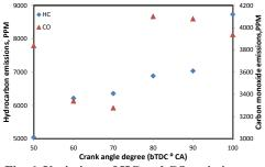
Fig. 6. Variations of HC and CO emissions at various single-pulse injection timings.
