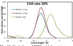
Fig. 19. Variations of HRR with boost pressures at the EGR rate of 30%.
