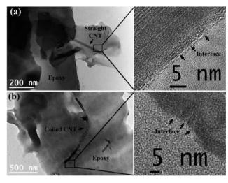
Fig. 5 High resolution bright field TEM images of nanocomposites reinforced with straight MWCNTs (a) and coiled MWCNTs (b) respectively. An individual CNT is spotted in both the cases to observe the interface. A continuous interlocked interface is observed in both nanocomposites.
