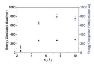
Fig. 9 The variation of energy dissipated and the energy dissipation rate in a DWCNT with different axial inner tube distances, S<sub>I</sub>, obtained from MD simulations.
