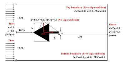
Figure 1: Computational domain with boundary conditions
