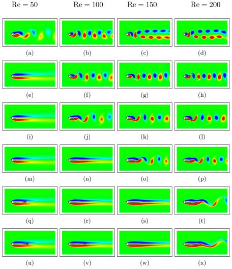
Figure 2: Instantaneous vorticity contours for an equilateral triangular cylinder attached with splitter plate of various lengths.(a-d) L = 0.0b, (e-h) L = 0.5b, (i-l) L = 1.0b, (m-p) L = 3.0b, (q-t) L = 5.0b, (u-x) L = 6.0b
