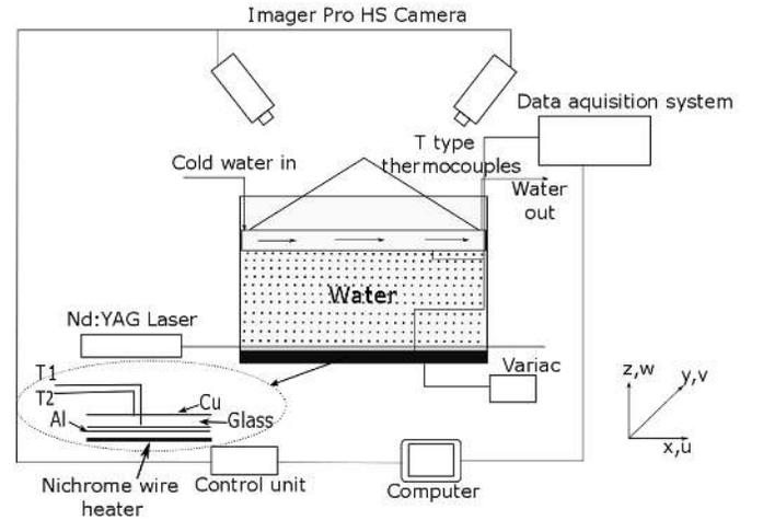
FIG. 2. Schematic of the experimental setup for steady RBC in water
