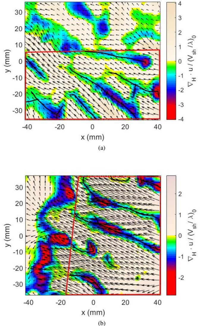
FIG. 3. Dimensionless horizontal divergence fields, overlaid over the horizontal velocity vector fields, in a horizontal plane at a height  $h_m$  from the hot surface in RBC in water. (a),  $Ra_w = 1.09 \times 10^8$ ,  $Re = 832$  and  $h_m = 1.5$  mm; (b),  $Ra_w = 6.03 \times 10^8$ ,  $Re = 2490$  and  $h_m = 1.3$  mm. Plumes are the colour regions. Shear dominant areas are shown by the red polygon.  $L_p$  is measured by adding up the length of the black lines in the plume regions.
