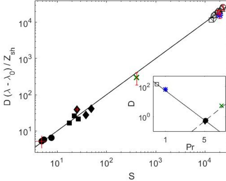
FIG. 7. Variation of  $\lambda^*$ , the difference of the mean plume spacing with shear ( $\lambda$ ) from the corresponding no-shear values ( $\lambda_0$ ), normalised by the viscous-shear length  $Z_{sh}$  (8), with the dimensionless shear parameter  $S$  (7); The symbols are as per figure 6 and table I; —, (14). The inset shows the variation of the prefactor  $D$  in (14) with  $Pr$ ; —, (15); ----, (16).
