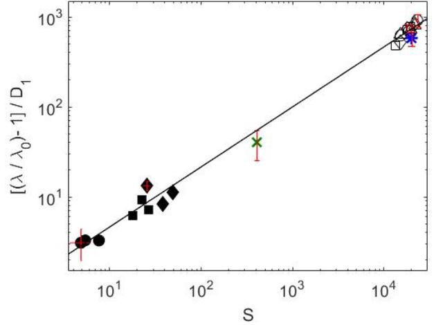
FIG. 8. Variation of the ratio of mean plume spacing with shear with the corresponding no-shear values with the dimensionless shear parameter  $S$  (7). The symbols are as per figure 6 and table I; —, (19).
