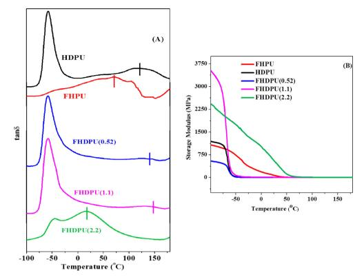
Fig. 8. (A) tand vs temperature (B) Storage modulus vs temperature plots of FHPU, HDPU and FHDPUs of their indicated Fe content. Plots in case of tand vs temperature are shifted vertically for better clarification.
