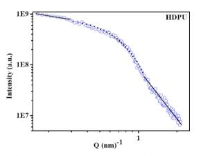
Fig. 9. Small angle X-ray scattering profile of HDPU. Solid line is representation of power-law. Dashed line is fit to the data.
