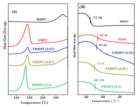
Fig. 7. DSC thermograms of FHPU, HDPU and FHDPUs of their indicated Fe %; in the temperature range: (A) 25–370 °C (B) – 100 °C to 25 °C.
