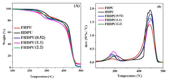
Fig. 6. (A) TGA and (B) DTG curve of FHPU, HDPU and FHDPUs(0.52-2.2).
