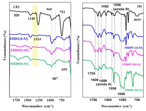
Fig. 1. FTIR spectra of (A) HTPB-DNB (HD) and PVF-g-HTPB-DNBs (FHD), (B) HTPB-DNB-PU (HDPU) and PVF-g-HTPB-DNB-PUs (FHDPU). Sample names are indicated in the figure. Amount of Fe content in the sample is mentioned in the parenthesis after the sample name.
