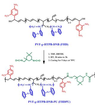
**Scheme 2.** Synthesis of PVF-g-HTPB-DNB (FHD) based polyurethanes (PU). These samples are abbreviated as FHDPU(XX) where XX indicate the Wt.% of Fe in the FHD samples.
