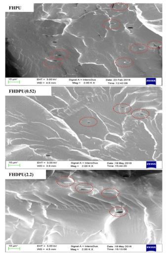
Fig. 11. FESEM images of the cross-section of cryo-fractured PU films: FHPU, FHDPU(0.52) and FHDPU(2.2).
