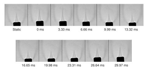
**Figure 7:** Instantaneous shadowgraphs of flames from static burner and burner vibrating with frequency 30 Hz and amplitude 1 mm ( $\Phi = 0.91$ ).
