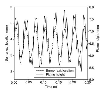
**Figure 11:** Time history of flame height oscillation and burner vibration for 30 Hz frequency and 1 mm amplitude.
