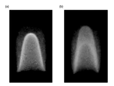
**Figure 4:** Naked eye view of typical (a) static and (b) vibrated flame.
