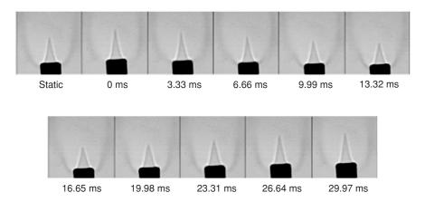
**Figure 6:** Instantaneous shadowgraphs of flames from static burner and burner vibrating with frequency 30 Hz and amplitude 1 mm ( $\Phi = 0.76$ ).
