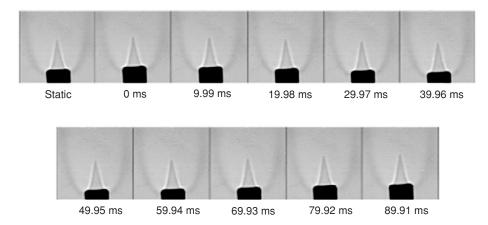
**Figure 5:** Instantaneous shadowgraphs of flames from static burner and burner vibrating with frequency 10 Hz and amplitude 1 mm ( $\Phi = 0.76$ ).
