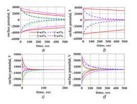
Fig. 12 Surface potential decay of gamma-irradiated epoxy nanocomposites
