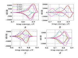
Fig. 13 Trap characteristics of gamma-irradiated epoxy nanocomposites a 0 kGy  $\,$
