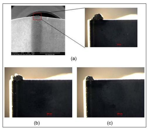
Figure 7. Built up edge formation for three different steels. (a) FP: 40 m/min, 0.125 mm/rev and 0.1 mm; (b) FBM: 40 m/min, 0.2 mm/rev and 0.1 mm; and (c) TM 40 m/min, 0.2 mm/rev and 0.1 mm.
