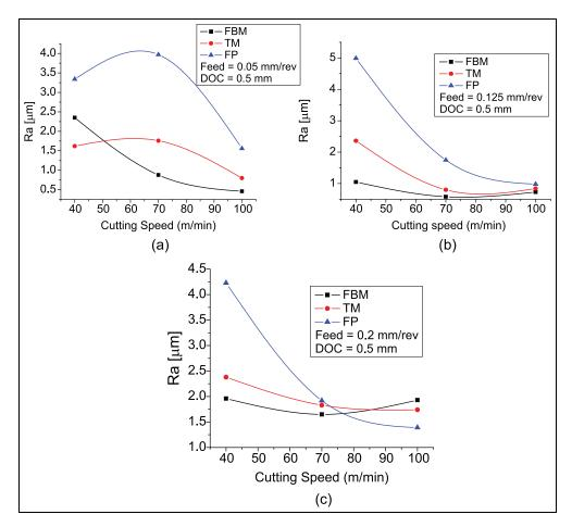
Figure 5. Surface roughness for different cutting speeds and feeds with constant depth of cut for (a) feed: 0.05 mm/rev, (b) feed: 0.125 mm/rev and (c) feed: 0.2 mm/rev.
