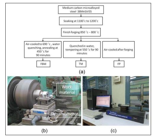
**Figure I.** (a) Thermomechanical processing sequence to obtain FBM, TM, FP microstructures, (b) VDF lathe fitted with Kistler dynamometer and (c) Mahr Perthometer.
