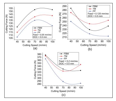
Figure 4. Cutting force obtained by varying cutting speed and feed with constant depth of cut: (a) feed: 0.05 mm/rev; (b) feed: 0.125 mm/rev; and (c) 0.2 mm/rev.
