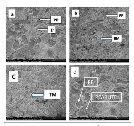
**Figure 2.** Scanning electron microscope microstructures for steel: (a) ferrite–pearlite, <sup>17</sup> (b) ferrite–bainite–martensite, <sup>18</sup> (c) tempered martensite and (d) as-received ferrite–pearlite microstructure.
