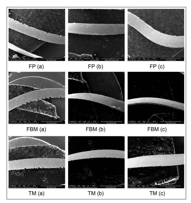
Figure 6. Chip formation for different feed rates. (a) 100 m/min, 0.2 mm/rev and 0.5 mm; (b) 100 m/min, 0.125 mm/rev and 0.5 mm; and (c) 100 m/min, 0.05 mm/rev and 0.5 mm.
