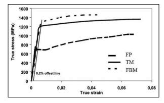
Figure 3. True stress and true strain plot for AC (FP), Q&T (TM) and TSCA (FBM).<sup>19</sup>.
