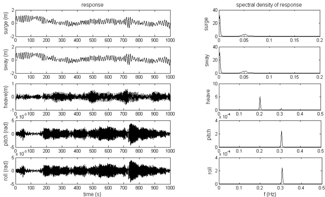
Fig. 5(a): Response of the TLP under the simulated North Sea freak wave ( $\alpha = 45^\circ$ ).
