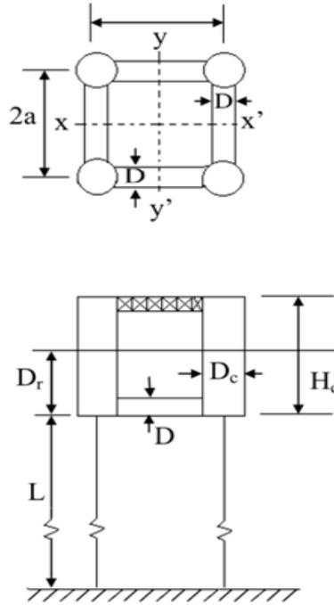
Fig. 3: Schematic plan and elevation of the TLP model.
