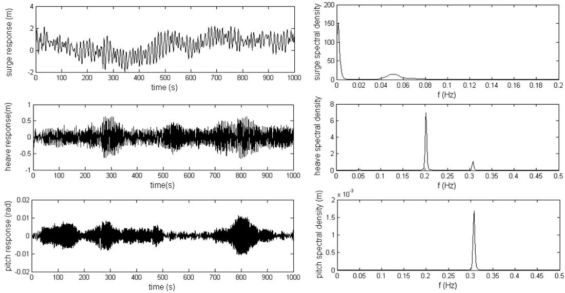
Fig. 4(b): Responses of the TLP for the simulated New Year wave ( $\alpha = 0^\circ$ ).
