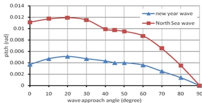
Fig. 7(e): Variation of the maximum response in pitch degree-of-freedom.
