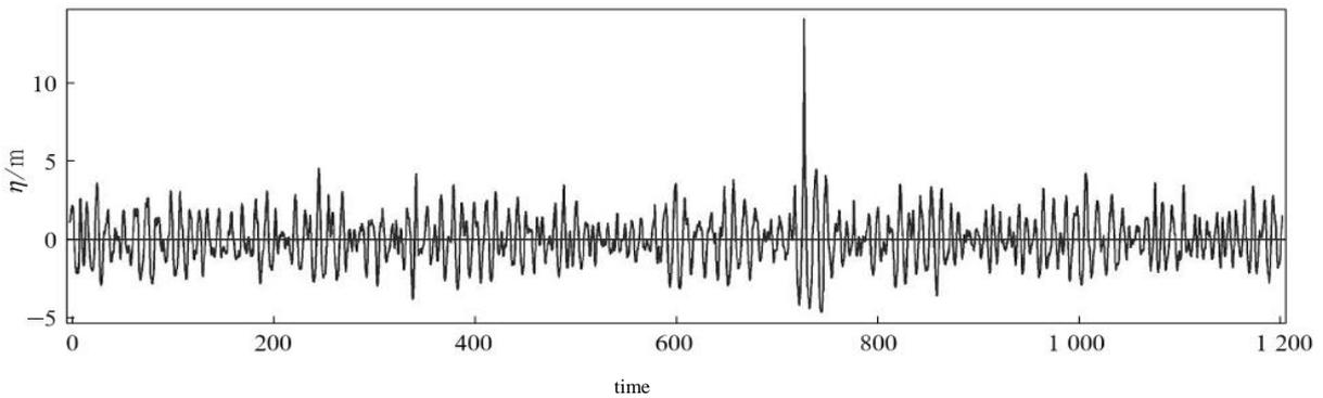
Fig. 2(a): Recorded time series of the North Sea freak wave.
