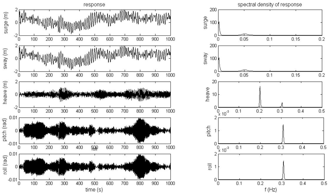
Fig. 5(b): Response of the TLP under the simulated New Year wave ( $\alpha = 45^\circ$ ).
