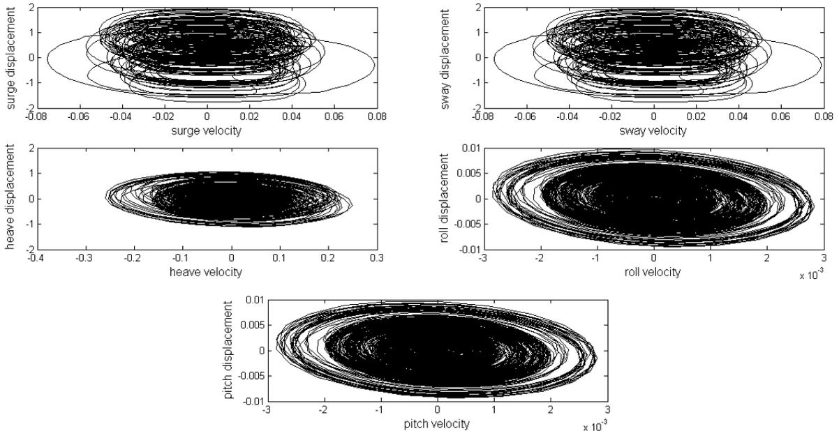
Fig. 6: Phase plots of the response of the TLP under simulated New Year wave ( $\alpha = 45^\circ$ ).
