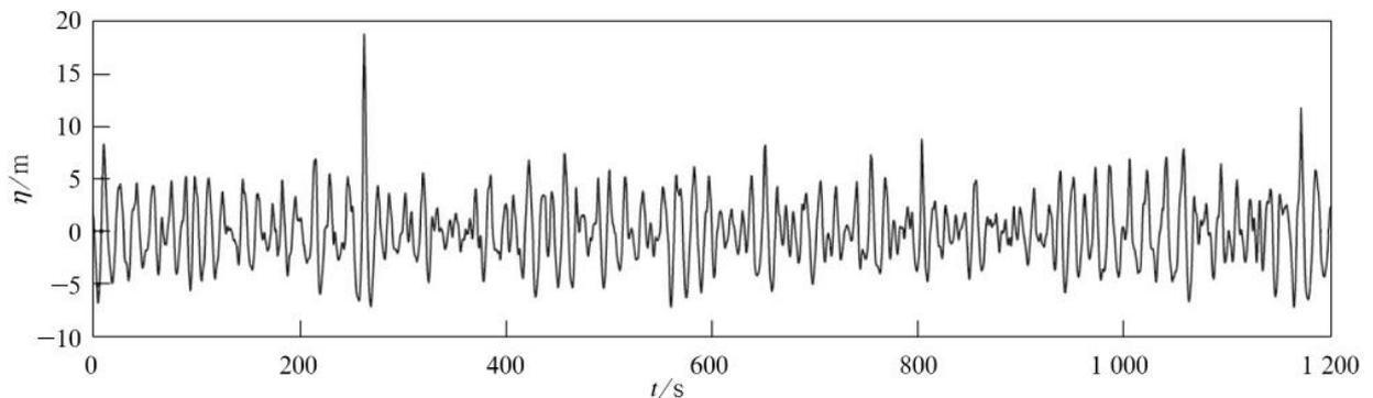
Fig. 1(a): Recorded time series of the New Year Wave at Draupner E platform.
