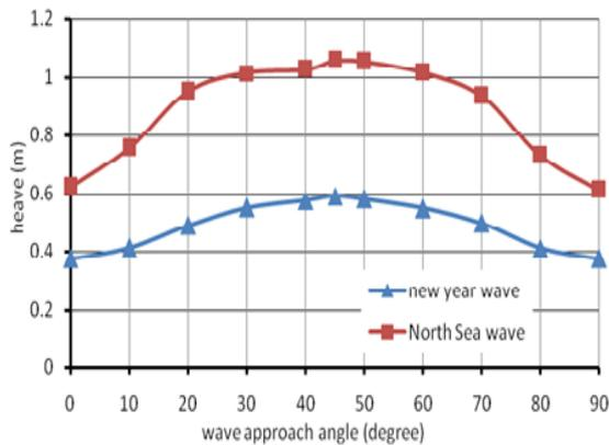
Fig. 7(c): Variation of the maximum response in heave degree-of-freedom
