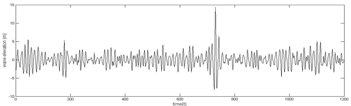
Fig. 2(b): Simulated time series of the North Sea freak wave.
