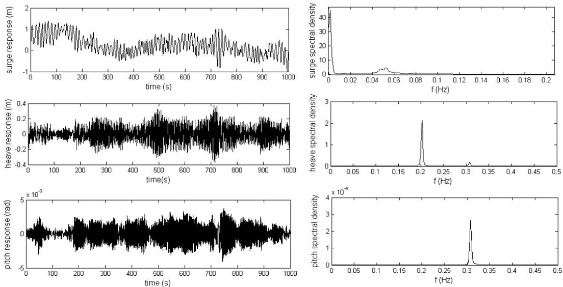
Fig. 4(a): Responses of the TLP for the simulated North Sea freak wave ( $\alpha = 0^\circ$ ).
