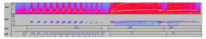
Figure 1: A sample illustrating the pre-processing and segmentation of audio. 1(a) Spectrogram of original audio while 1(b) Spectrogram after pre-processing the audio. 1(c) Labeled ground-truth for the audio. Figure 1(d) output obtained from GD based segmentation algorithm.
