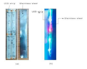
Fig. 2. Stainless steel cantilever sensor : (a) sensor unit with front and reverse view; (b) side view of sensor inserted inside pipe. LED strip and camera are used to capture the deflection of the strip as a function of the flow to evaluate the proposed cantilever based scheme.
