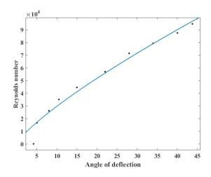
Fig. 8. Non-dimensional plot of angle of deflection vs Reynolds number
