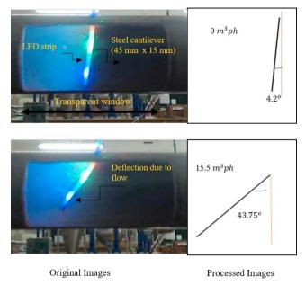
Fig. 6. Original images captured from the camera and processed images with angle from the algorithm. 4.2 <sup>o</sup> offset is present in the prototype, due fixed the mechanical misalignment.
