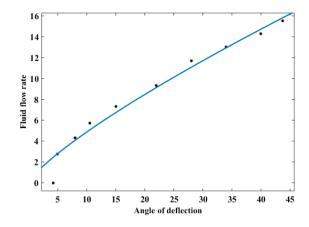
Fig. 7. Calibration model for flow rate and angle of deflection.
