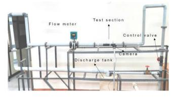
Fig. 3. Experimental system with the prototype flow sensor and a flow meter to compare the results.
