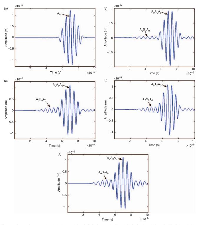
**Figure 2.** A-scans from numerical simulations on  $[0/\pm 45/90]_s$  laminate: (a) with no delamination (intact), (b) with delamination interface between plies 0, +45, (c) +45, -45, (d) -45, 90, and (e) 90, 90.
