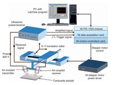
Figure 3. Schematic of experimental set up.
