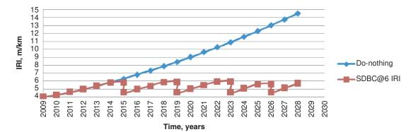
FIGURE 6 Comparison of roughness progression for doing nothing and maintenance with semidense bituminous concrete (SDBC) at 6 IRI.
