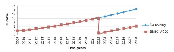
FIGURE 8 Comparison of roughness progression for doing nothing and maintenance with BM50 + asphalt concrete (AC) 20 at 10 IRI.
