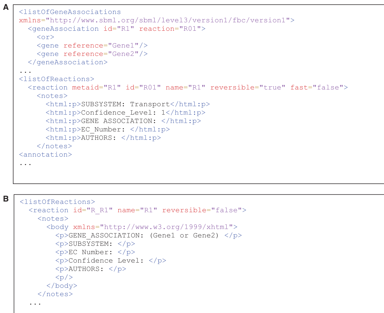
Figure 2. Different types of representations of Gene Protein Reaction Association in SBML format: Panel A illustrates how the gene-protein-reaction associations are specified in Flux Balance Constraints package, while Panel B illustrates the same in COBRA Format. Note that the FBC package, in addition to the geneAssociation field, consists of a separate notes field, which contains the details about the GPRs involved in the given reaction.
