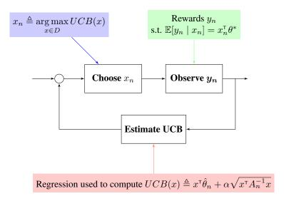
Figure 5: Operational model of LinUCB
