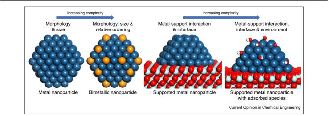
Schematic illustration of the structure of a metallic nanoparticle, bimetallic alloy nanoparticle, metal nanoparticle supported on metal oxide and metal nanoparticle supported on metal oxide containing adsorbed species from the reaction environment.
