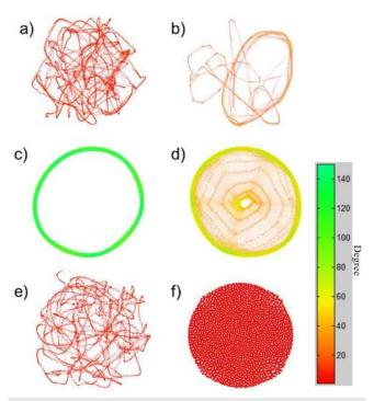
**FIG. 13.** Recurrence networks corresponding to combustion noise [(a) and (e)], intermittency [(b) and (d)], and thermoacoustic instability (c). (f) corresponds to a network of random noise. The color of the node represents the degree of the node. Image reproduced with permission from Godavarthi *et al.*, "Recurrence networks to study dynamical transitions in a turbulent combustor," Chaos **27**, 063113 (2017). Copyright 2017 AIP Publishing LLC.
