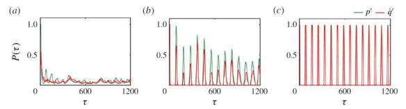
**FIG. 8.** Probability of recurrence,  $P(\tau)$ , for both p' and q' during (a) combustion noise (DS), (b) weak thermoacoustic instability (PS), and (c) strong thermoacoustic instability (GS). Reproduced with permission from Pawar *et al.*, "Thermoacoustic instability as mutual synchronization between the acoustic field of the confinement and turbulent reactive flow," J. Fluid Mech. **827**, 664–693 (2017). Copyright 2017 Cambridge University Press.
