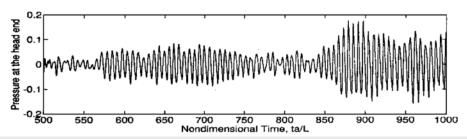
FIG. 4. Time series of unsteady pressure corresponding to thermoacoustic oscillation, resulting from the influence of stochastic fluctuations on a deterministic model as described by Burnley and Culick.<sup>32</sup> Reproduced with permission from V. Burnley and F. C. Culick, "Influence of random excitations on acoustic instabilities in combustion chambers," AIAA J. 38, 1403-1410 (2000).
