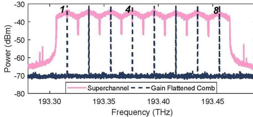
Fig. 7. Spectrum of the 8 channel 608 Gbps 16QAM CO-OFDM superchannel.
