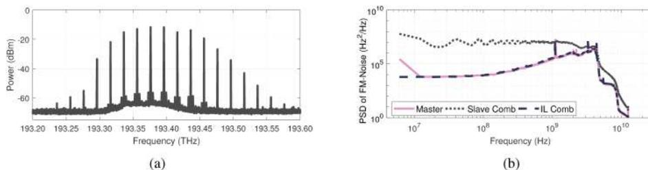
Fig. 3. (a) Output spectrum of the injection locked gain-switched comb (b) FM-noise spectrum of the master laser and that of a comb line before and after the injection.
