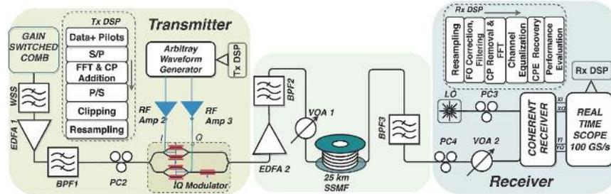
**Fig. 4.** Schematic of the experimental setup to perform the transmission of 16/32/64QAM CO-OFDM with injection locked gain switched comb.
