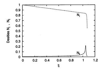
FIG. 12. Density profile of ions and dust grains in the whole plasma for case II. The dust density shows the formation of a steep structure as the dust slows down. Dust values are raised by an order  $10^8$  to plot it together with ion plot.
