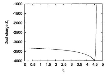
FIG. 9. Charge on dust grains  $Z_I$  plotted vs  $\xi$  for case I. The charge shows an increase in the presheath region and then a sharp decrease in the sheath region.
