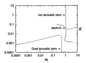
FIG. 4. Root locus of solutions for the third case where the dust grains are coupled strongly to the plasma. The dashed lines indicate the ion-acoustic and the dust-acoustic presheath singularities. The solid line indicates the evolution of the solution in  $M_i$ - $M_I$  space for a case where the ion velocity builds up to its singular value and at the same time the dust velocity shows interesting features of stagnation towards the sheath edge.
