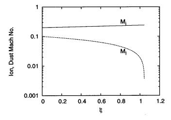
FIG. 10. Velocity profile of ions and dust grains in the presheath region for case II (plotted on a log scale). The dust grains show a drop in flow velocity (dashed curve) and ions show no appreciable change in flow velocity (solid curve).
