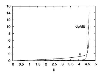
FIG. 8. Potential ( $\psi$ ) and electric field ( $d\psi/d\xi$ ) profiles for case I.  $\psi$  profile is monotonic. Electric field also show standard sheath features.
