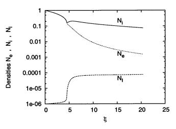
FIG. 15. Density profiles of electrons, ions, and dust grains for case III. The dust density rises, the electrons density drops faster than the ion density.
