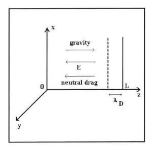
FIG. 1. Model system under consideration. z=0 defines the beginning of the presheath and z=L is the position of the wall.
