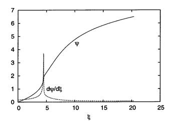
FIG. 17. Nonmonotonic potential profile for case III. Electric field profile shows the formation of a nonlinear structure.
