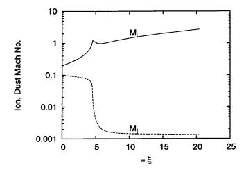
FIG. 14. Velocity profile of ions and dust grains for case III. The ions profile (solid curve) shows a kink at the point when the dust velocity (dashed curve) drops sharply. The dust flow flattens as it reaches the wall.
