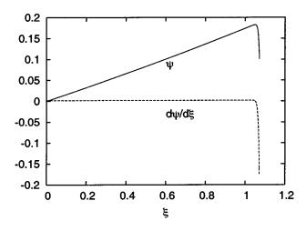
FIG. 13. Potential and electric field shows a sign reversal in case II.
