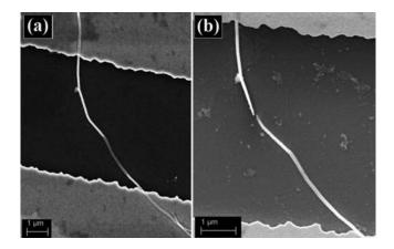
FIG. 1. SEM image of MWNT (a) lying on two gold electrodes, separated by dielectric  $SiO_2$ , (b) same tube after current induced breakdown.
