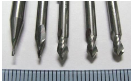
Figure 3. Micro-milling tools, from left to right: straight tool, 15°, 30°, 40° and 50° tapered tools.
