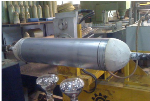
Figure 2: Steel mandrel with POP end domes ready for winding
