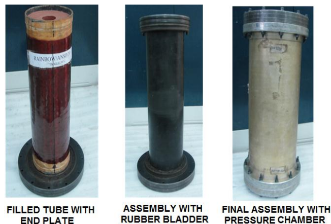
Figure 8: Stages of assembly of hardware for testing
