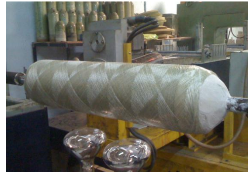
Figure 3: Glass epoxy tube under winding using S2 glass tow prep
