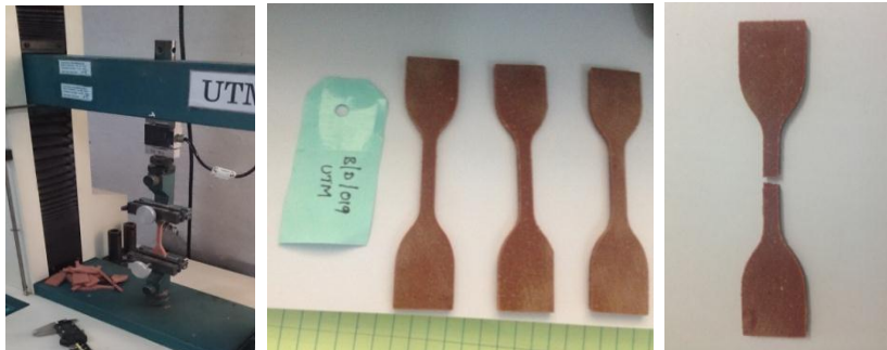
Figure 4: Inert propellant sample under uni-axial testing as per ASTM D638
