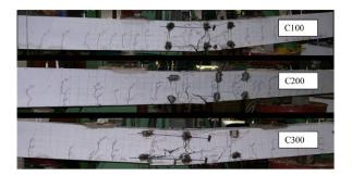
Figure 8. Formation of cracks in coated beams.
