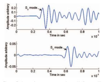
Figure 7. A-scans from experiments, taken at (a) "Receiver I" and (b) "Receiver 2" across fiber direction.
