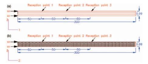
Figure 3. Specification of model used for FE simulations. Excitation of So mode (a) along fibers and (b) across fibers.
