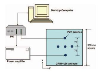
Figure 4. Schmatic of experimental set up.
