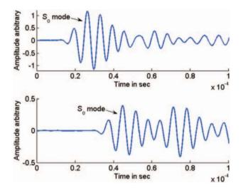
Figure 6. A-scans from experiments, taken at (a) "Receiver I" and (b) "Receiver 2" along fiber direction.
