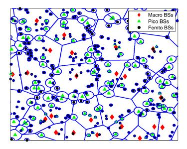
Fig. 1. A realization of a Poisson distributed three-tier cellular network with coverage regions defined by the highest received power.
