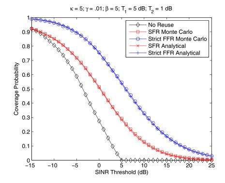
Fig. 4. Downlink edge user SINR distributions for open access with two tiers of APs.
