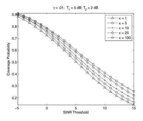
Fig. 5. Downlink edge user SINR distributions for Strict FFR and closed access as a function of the tier density ratio  $\kappa$ .
