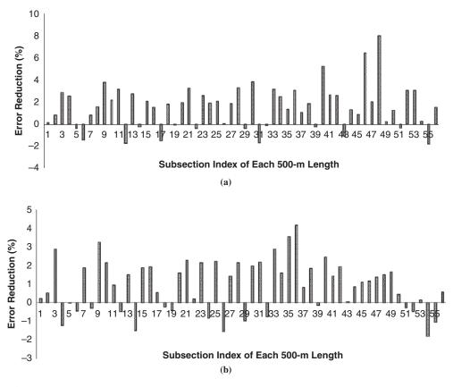
FIGURE 5 Error reduction by considering previous two subsections rather than previous one subsection for (a) off-peak trips and (b) peak trips.
