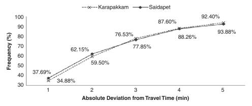
FIGURE 6 Results of predicted arrival time deviation at selected bus stops.
