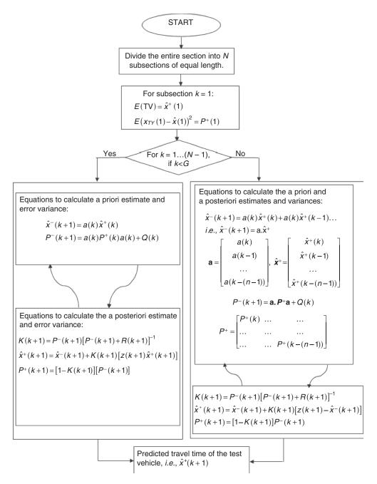
FIGURE 2 Flowchart representing the proposed method (E = expected travel time; TV = test vehicle;  $\hat{x}$  = travel time; K = Kalman gain; P = error variance; z = latest available measurement from the field; - and + in superscript = a priori and a posteriori estimates, respectively).
