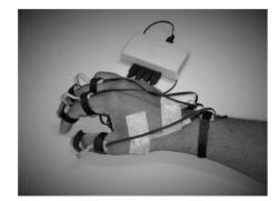
FIG. 3. i-Glove designed for hand rehabilitation/assessment.
