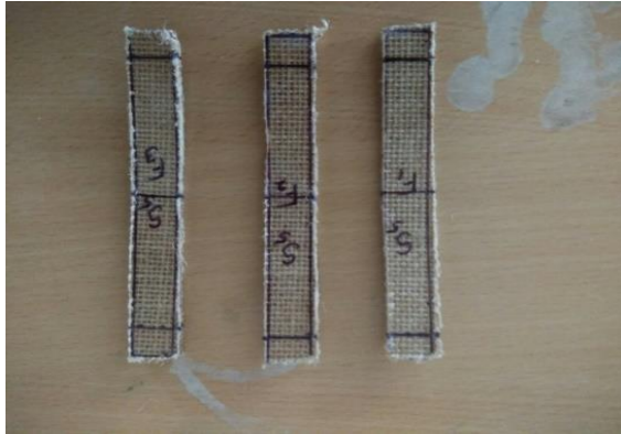
Figure 12: JS5 Tensile Specimen Failure Pattern
