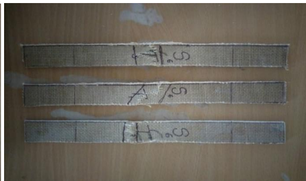
Figure 10: JS6 Tensile Specimen Failure Pattern
