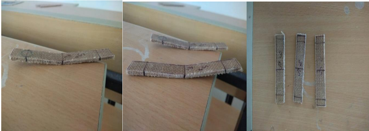
Figure 16: JS4, JS7, FS2 Flexure Specimen Failure Pattern
