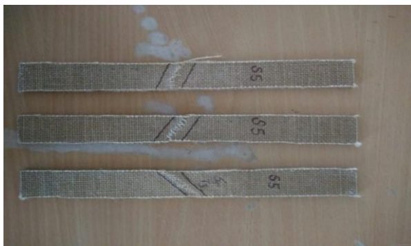
Figure 9: JS5 Tensile Specimen Failure Pattern
