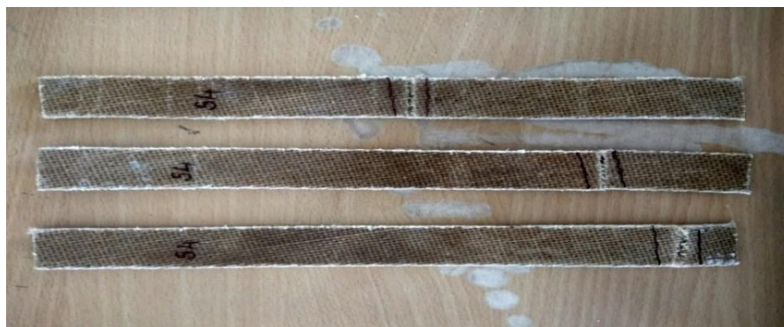
Figure 5: JS4 Tensile Specimen Failure Pattern
