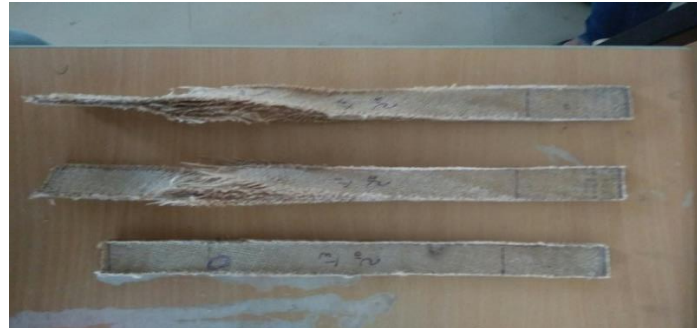
Figure 7: JS10 Tensile Specimen Failure Pattern
