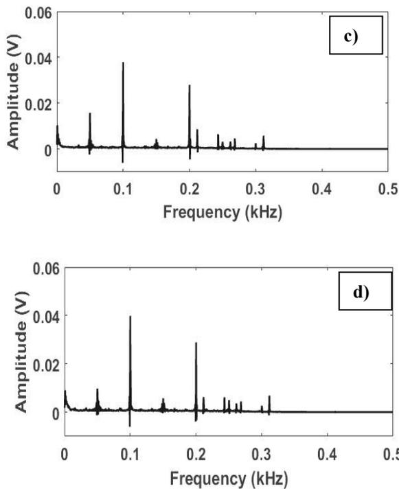
Fig. 7. Vibration FFT analysis during initial cutting pass
