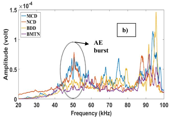
Fig.6. AE FFT analysis during machining a) Initial cutting pass b) Final cutting pass
