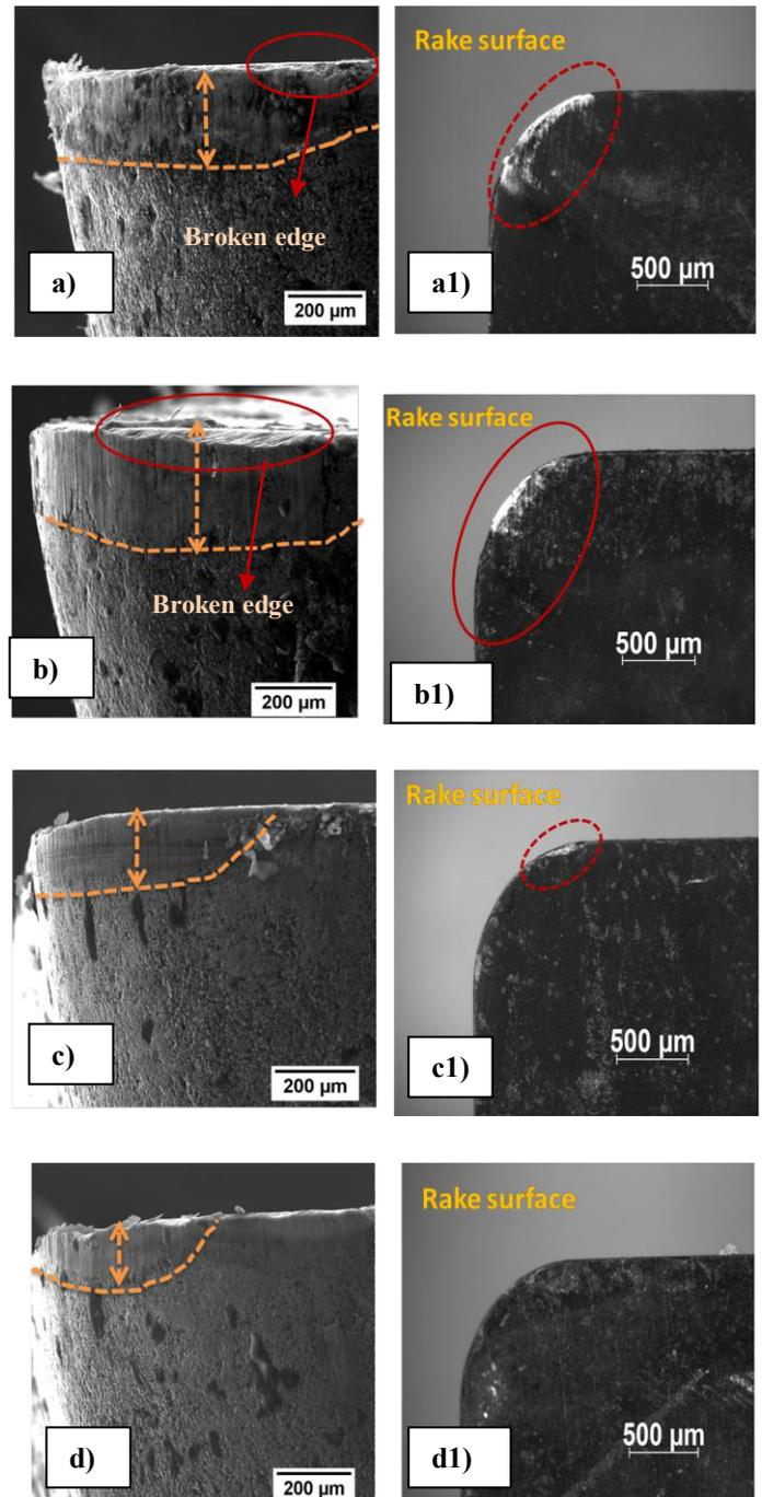
Fig. 4. SEM (a,b,c,d) and Stereo microscopic (a1,b1,c1,d1) image of cutting tool after final cutting pass
