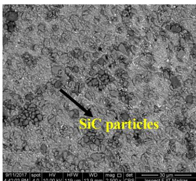
Fig. 1. Microstructure of Al-SiC MMC
