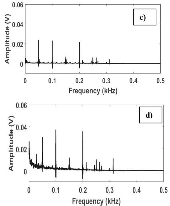
Fig. 8. Vibration FFT analysis during final cutting pass
