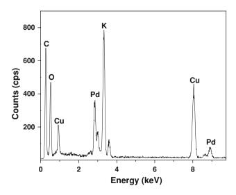
Fig. 6 EDAX spectrum of intermediate complex, K<sub>2</sub>[Pd(C<sub>2</sub>O<sub>4</sub>)<sub>2</sub>]
