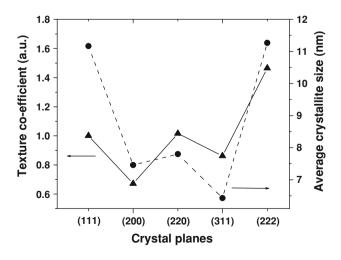
Fig. 3 Average crystallite size and texture coefficient of Pd nanoparticles calculated from XRD powder pattern
