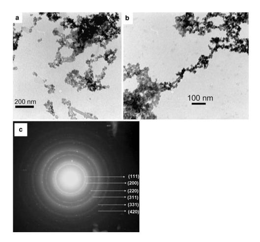
**Fig. 1 a, b** TEM images of Pd nanoparticles synthesized by photochemical decomposition method; c SAED pattern recorded on aggregates of Pd nanoparticles (111)
