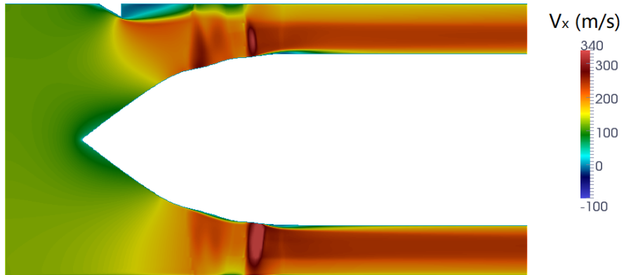
(a) Axial velocity distribution on the meridional plane
