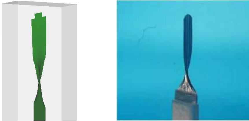
(a) Predicted failure surface from the proposed local crack-tracking approach (b) Experimentally observed failure surface from Citarella and Buchholz [59]
