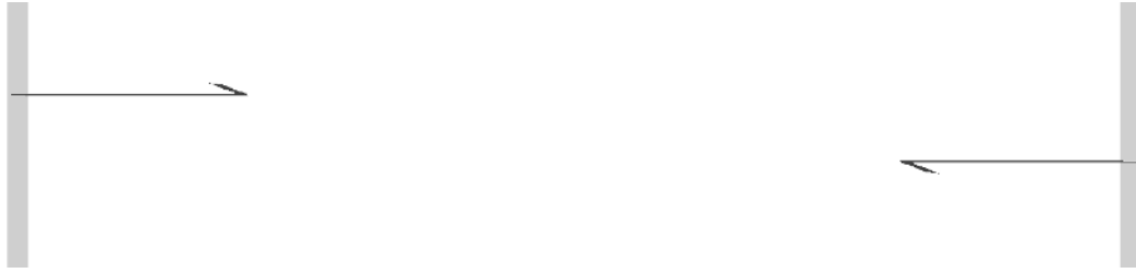
(b) Predicted crack path from the global algorithm with cracks initiated at y = 18.81 and y = 21.19 . Thermal boundary conditions are applied on the nodes of cut elements and on the edges: \mathcal{S}^1, \mathcal{S}^2, \mathcal{S}^3 , and \mathcal{S}^4
