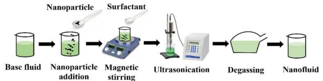
Figure 2. Two-step method for preparation of nanofluids.
