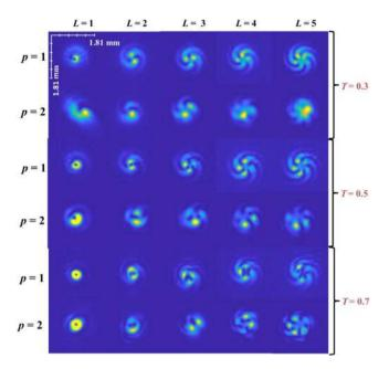
**Figure 5.** Recorded intensity patterns at plane  $f_2$  with the scatterer at  $f_1$ . The first rows present the results for one (p=1) and two (p=2) scatterers, whereas the columns are the results for the topological charges L=1 to 5. The experimental results for different splitting ratios (T=0.3, 0.5 and 0.7) are presented in subsequent rows.
