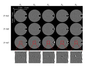
**Figure 2.** Images of MDOEs for different topological charges L=1 to 5 and splitting ratios T=0.3, 0.5 and 0.7 designed with two-phase levels and a linear phase of  $\alpha=0.03$  radians. The number of lines in the fork pattern increases with the topological charges.
