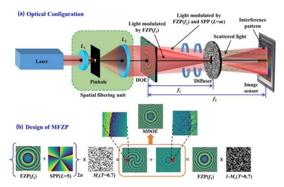
**Figure 1.** (a) Optical configuration of the single channel, dual beam interferometer. The light from the laser is spatially filtered and collimated by a pinhole and refractive lenses  $L_1$  and  $L_2$ . (b) Technique by which the MDOE is designed.
