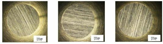
Fig. 3 Wear scar optical images of brass pin samples for (a) 10N, (b) 20N and (c) 30N loads
