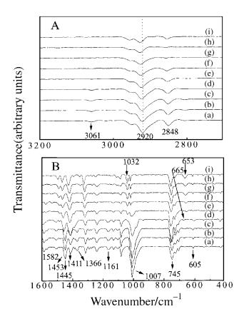
**Fig. 6** Variable temperature FTIR spectra for AuMBT in (A) the high wavenumber and (B) the low wavenumber region. The temperatures are: (a) 298, (b) 323, (c) 348, (d) 373, (e) 398, (f) 423, (g) 448, (h) 473 K and (i) cooling back to 298 K, respectively.
