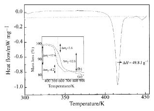
**Fig. 7** Differential scanning calorimetric traces of AuMBT. The full line (—) represents heating cycle and the dashed line shows the cooling cycle (---). The enthalpy of transition is indicated. The inset shows TGA curves of (a) AuMBT and (b) AgMBT. Mass losses are indicated.
