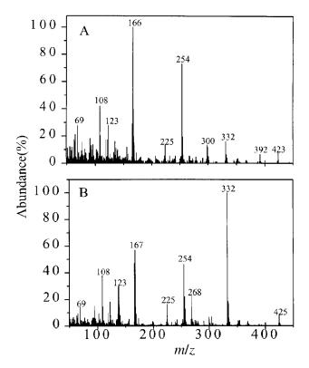
**Fig. 3** Mass spectra of (A) AgMBT and (B) AuMBT. Peaks of interest are marked. Assignments of the peaks with possible structures are given in Table 1.
