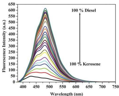
**Fig. 5** WLEF spectra of diesel–kerosene mixtures measured using the fiber optic fluorimeter (FOF) instrument.
