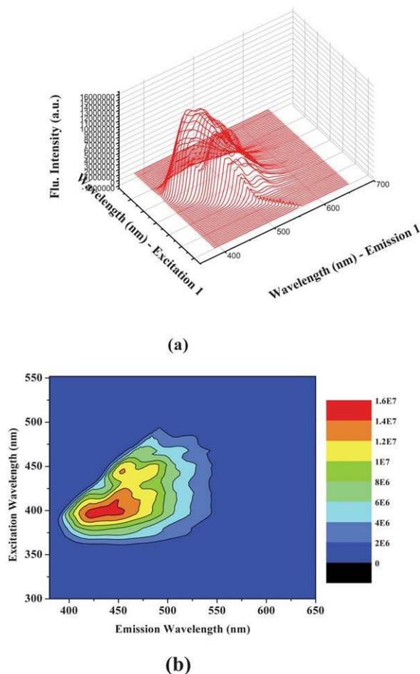
Fig. 3 (a) 3-D and (b) contour plot of pure diesel.
