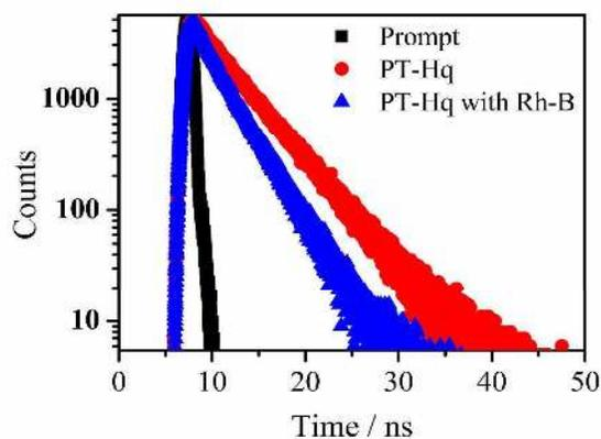
Figure 10. Fluorescence decay curves of pure PT-Hq ( $10^{-5}$  M in THF) and PT-Hq with Rh-B ( $10^{-5}$  M in water)
