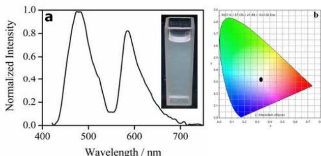
**Figure 4.** (a) Emission spectrum of mixture of **FL-E** (1 mL of  $10^{-5}$  M, in THF), **PT-Hq** (1 mL of  $10^{-5}$  M, in THF) and **Rh-B** (1 mL of  $10^{-5}$  M, in water) in solution state, excited at 411 nm. Inset shows the photograph of corresponding white light under UV excitation. (b) CIE diagram of the corresponding white light emission in solution state.
