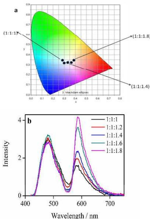
**Figure 5.** (a) CIE chromaticity diagram obtained on changing the volume of **Rh-B** from 1 mL to 1.8 mL, while keeping the volume of **FL-E** and **PT-Hq** at 1 mL each. (b) The corresponding fluorescence titration spectra.
