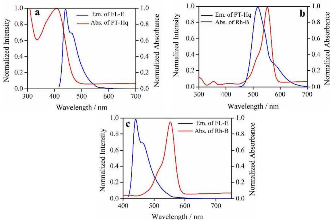
**Figure 8.** (a) Spectral overlap of fluorescence spectra of FL-E (blue) and absorption spectra of PT-Hq (red); (b) Spectral overlap of fluorescence spectra of PT-Hq (blue) and absorption spectra of Rh-B (red); (c) Spectral overlap of fluorescence spectra of FL-E (blue) and absorption spectra of Rh-B (red).
