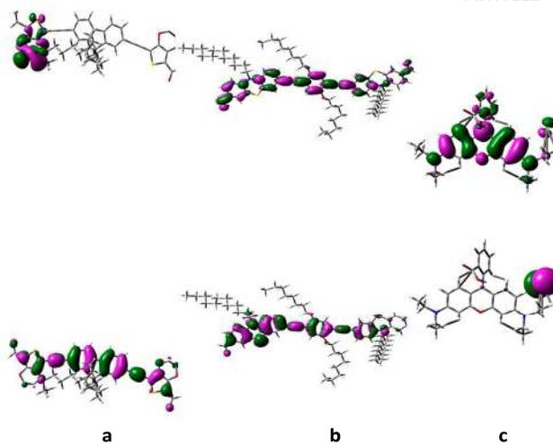
Figure 12. B3LYP/6-31G<sup>\*</sup> DFT calculated HOMO (bottom) and LUMO (top) contours of (a) **FL-E** (b) **PT-Hq** and (c) **Rh-B**. The decrease in energy band gap from (a) to (c) is approximate (not drawn to the scale).
