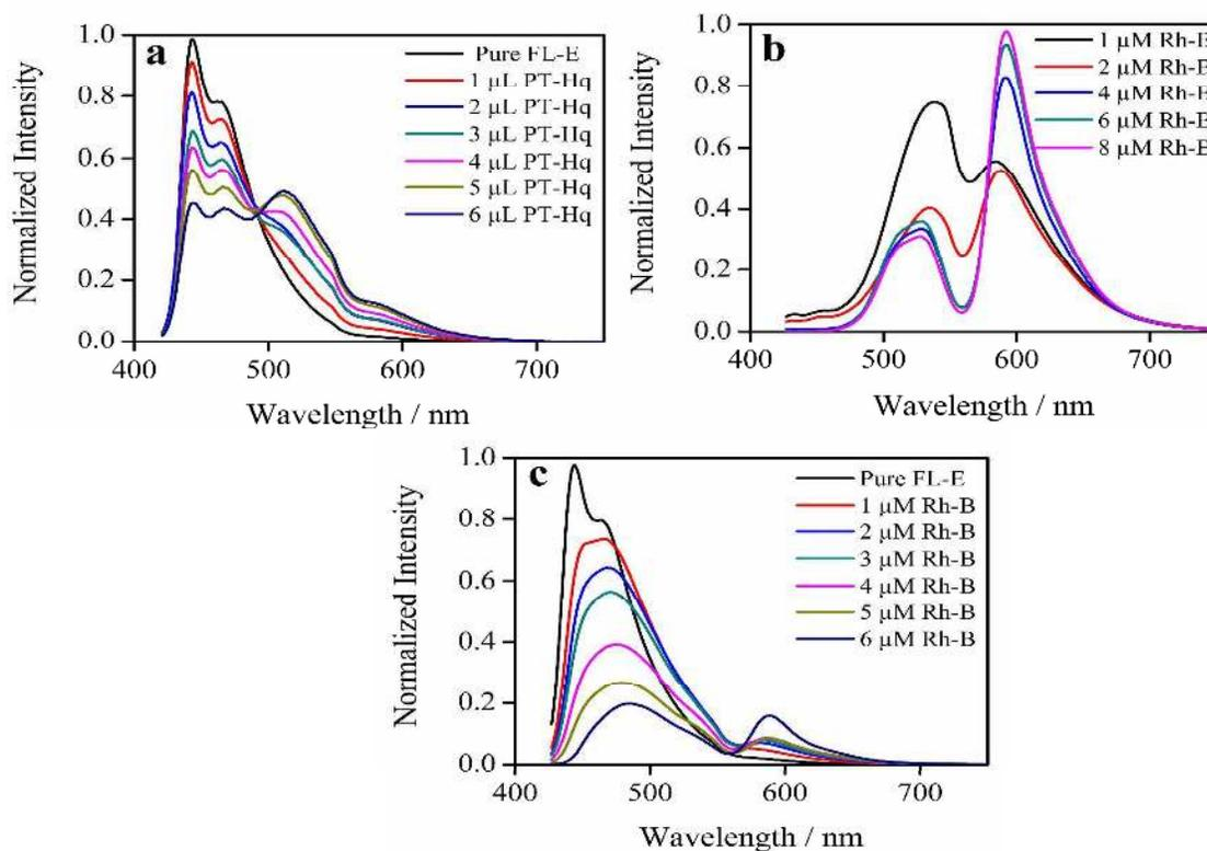
**Figure 9.** (a) Fluorescence spectra of FL-E ( $10^{-5}$  M, in THF) with the addition of PT-Hq (in THF) excited at 411 nm. (b) Fluorescence spectra of PT-Hq ( $10^{-5}$  M, in THF) with the addition of Rh-B (in water) excited at 411 nm. (c) Fluorescence spectra of FL-E ( $10^{-5}$  M, in THF) with the addition of Rh-B (in water) excited at 411 nm.
