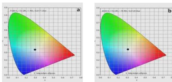
**Figure 7.** (a) CIE diagram of the corresponding white light emission in PMMA film. (b) CIE diagram of the corresponding white light emission in gelatin gel
