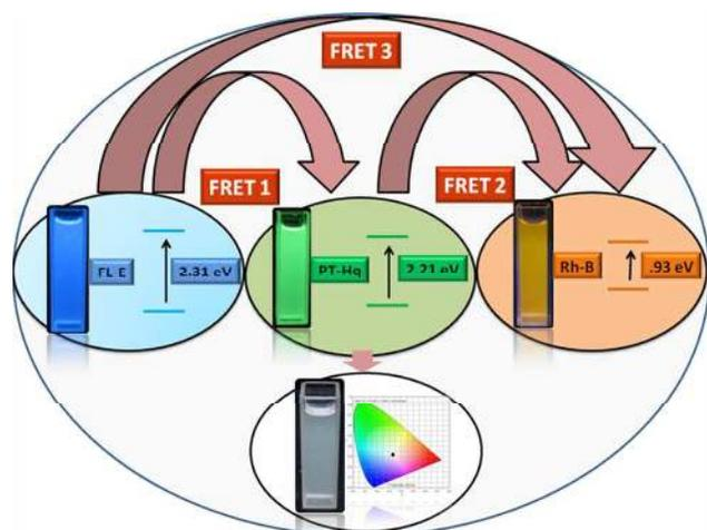
Scheme 2: Schematic presentation of FRET for the molecules FL-E, PT-Hq and Rh-B in solution along with their approximate energy level diagrams.
