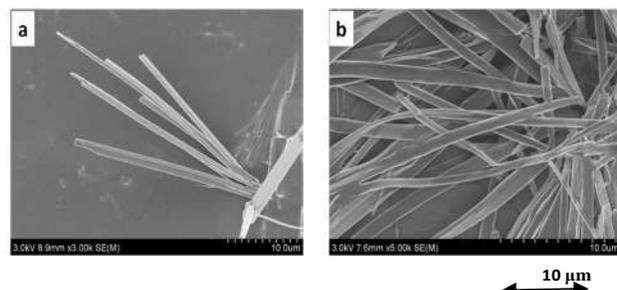
**Figure 1.** SEM images of (a) FL-E and (b) PT-Hq both showing fibrous alignment
