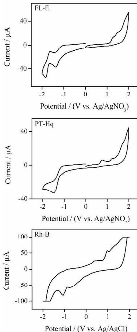
Figure 11. Cyclic voltammograms of FL-E, PT-Hq and Rh-B in solution state, 0.2 M Bu<sub>4</sub>NPF<sub>6</sub> as supporting electrolyte for FL-E and PT-Hq while 0.1 M KNO<sub>3</sub> as supporting electrolyte for Rh-B.
