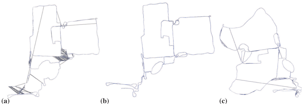
Figure 8. (a) The input dataset named Bovisa04. Bovisa04 dataset is available in RAWSEEDS (RAWSEEDS 2009). (b) The output of robust SLAM back-end algorithm RRR (Latif et al 2012a, 2013). It is able to reject wrong loop closures. The source code of RRR algorithm and input dataset are taken from author's website (Latif 2014). (c) Output of plain SLAM back-end. This output is generated using implementation of Gauss-Newton algorithm in g^2o (Kümmerle et al 2011) library. The source code of g^2o is available at author's website (Kuemmerle 2014).
