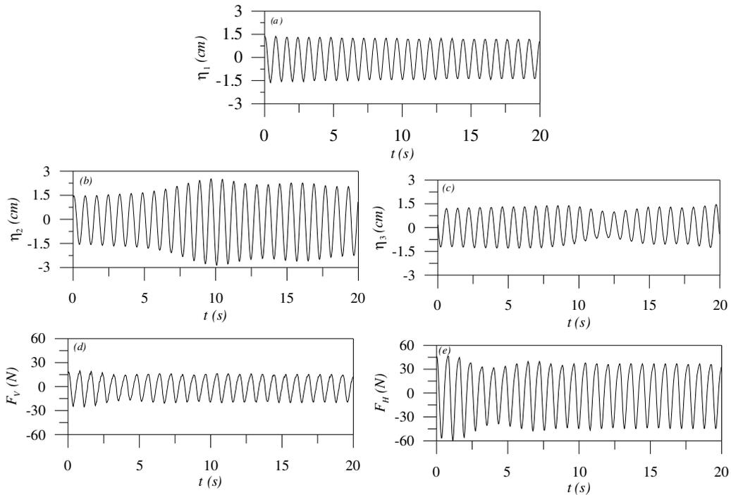
Fig. 3. Typical time histories of (a)  $\eta_1$ , (b)  $\eta_2$ , (c)  $\eta_3$ , (d)  $F_V$ , (e)  $F_H$  circular curve bottom OWC. ( $H/L=0.0302$  and  $d/L=0.5018$ )
