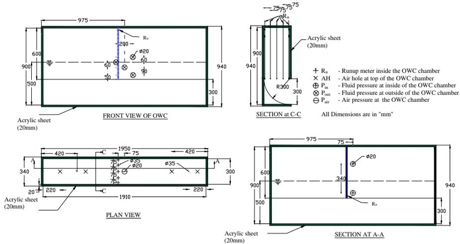
Fig. 2. Dimensional details of OWC
