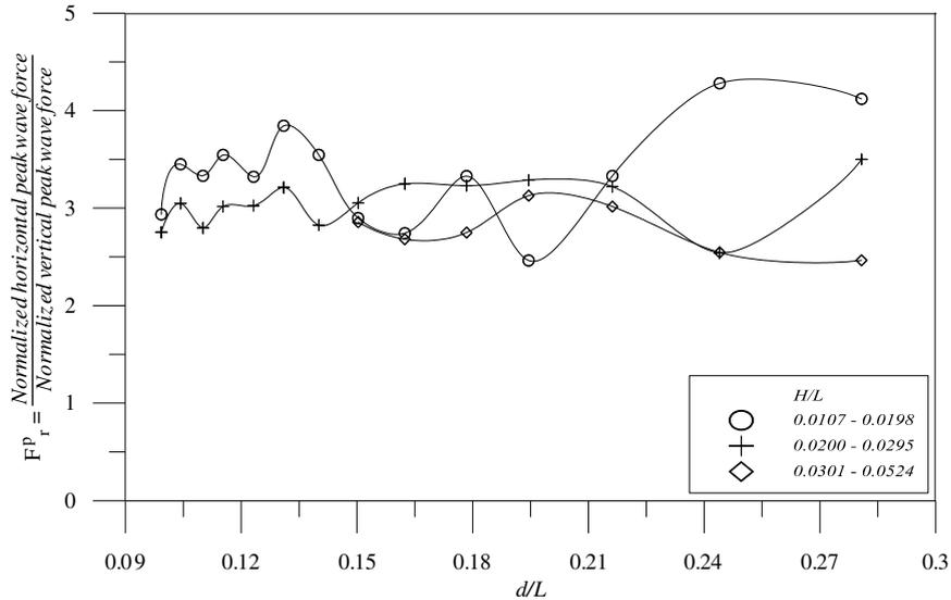
Fig. 6 Variation of normalized peak wave force ratio with d/L (for different H/L range)
