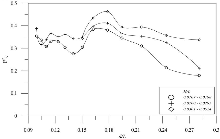
Fig. 4. Variation of normalized vertical peak wave force with  $d/L$  (for different  $H/L$  range)
