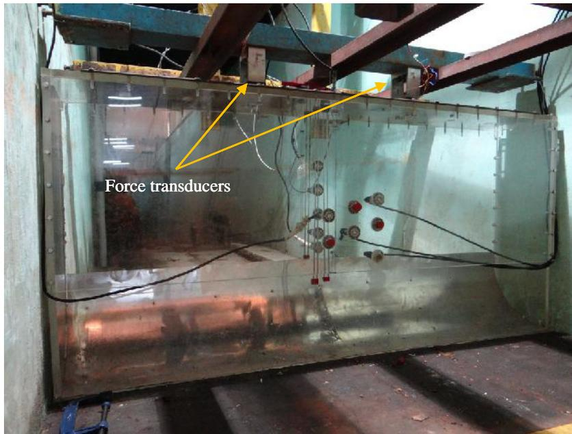
Fig. 1b. The force transducer arrangement details.
