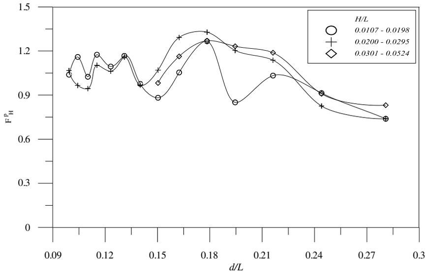
Fig. 5 Variation of normalized horizontal peak wave force with d/L (for different H/L range)
