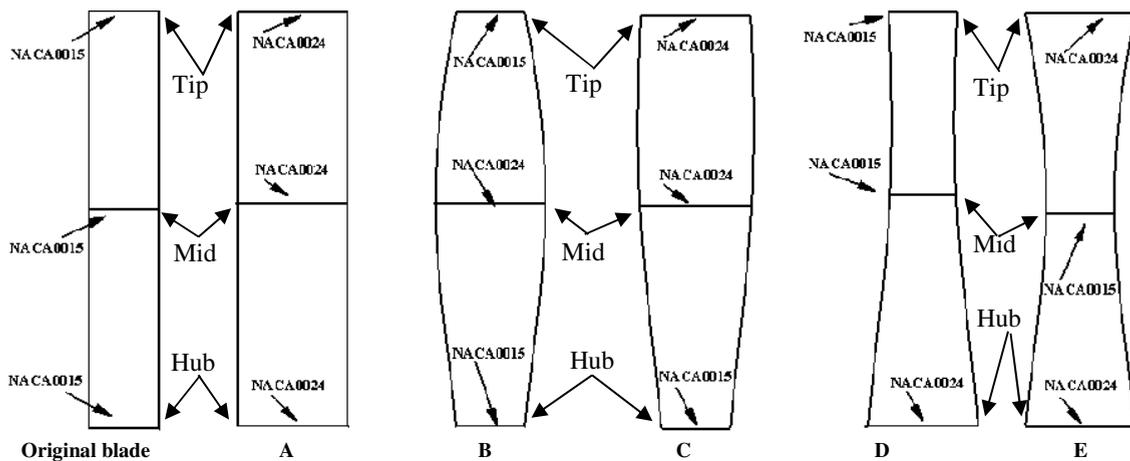
Fig. 1. Variation of blade profile thickness from hub-to-tip
