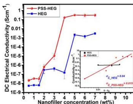
**Figure 5.** Electrical conductivity of the PVDF/HEG and the PVDF/PSS-HEG with varying concentrations. Inset figure shows the relationship between  $(\phi - \phi_c)$  and conductivity of HEG and PSS-HEG in the PVDF polymer matrix.
