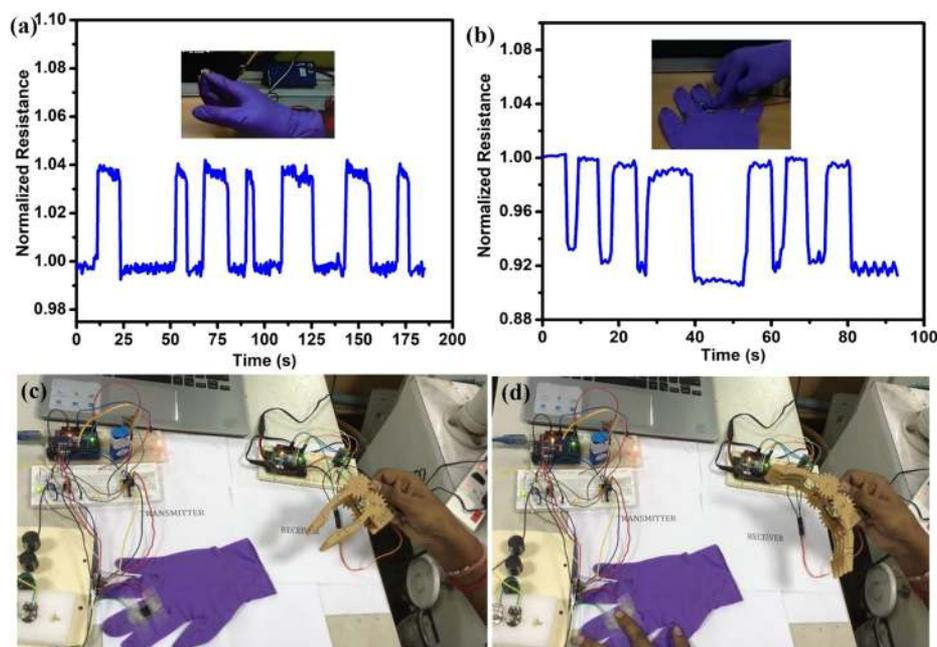
**Figure 9.** Demonstration of the flexible strain sensor for wearable device applications. (a) Finger bending and (b) pressing. Controlling of robotic arm using the strain sensor (c) unstrained and (d) strained positions.
