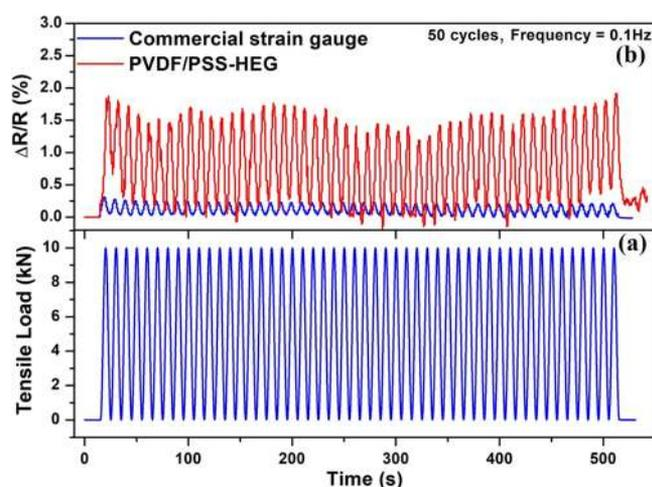
**Figure 7.** (a) Applied tensile cyclic load of 10 kN for 50 cycles with a frequency of 0.1 Hz and (b) response of the PVDF/PSS-HEG-1.5 wt %-based flexible strain sensor and commercial metallic strain gauge for the applied cyclic loading.
