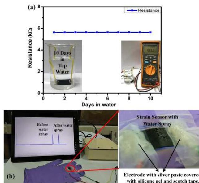
**Figure 8.** (a) Electrical resistance of the flexible strain sensor, which is immersed in water over the period of 10 days. (b) Response of the flexible strain sensor for the applied strain before and after the water spray, and inset figure shows the zoomed-in view of the presence of water droplets on the strain sensor.
