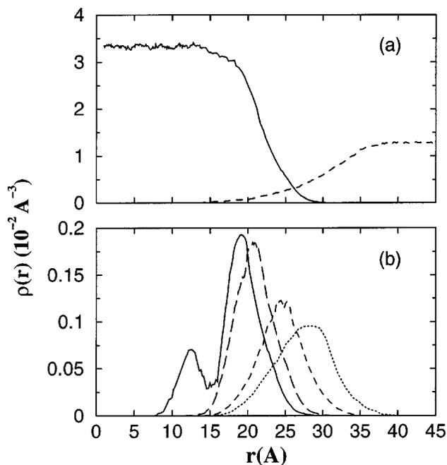
FIG. 2. The number density profile of (a) water (solid line) and carbon dioxide (dashed line) and (b) sodium (solid line), head group phosphorus (long dashed line), tail CH<sub>2</sub> (short dashed), and tail CH<sub>2</sub> (dotted line) as a function of the distance from the center of the aqueous core.
