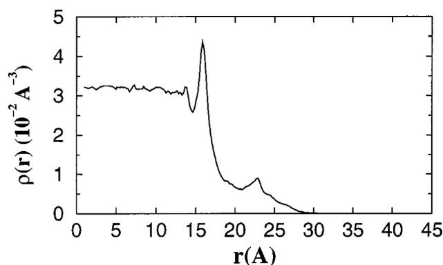
FIG. 3. The number density profile of water with respect to the effective surface formed by the head group phosphorous atoms.
