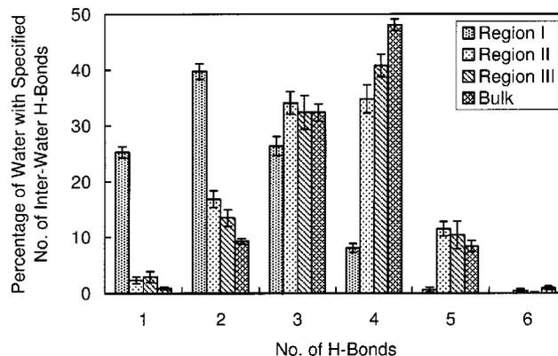
FIG. 5. The distribution of interwater hydrogen bonds for water in the three regions along with the distribution for bulk water. The *x*-axis denotes the number of hydrogen bonds per water molecule and the *y*-axis denotes the percentage of water with that many number of H bonds.
