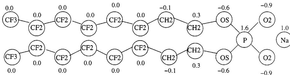
FIG. 1. Structure of the fluorosurfactant molecule. The numbers are the values of the atom-centered point charges.
