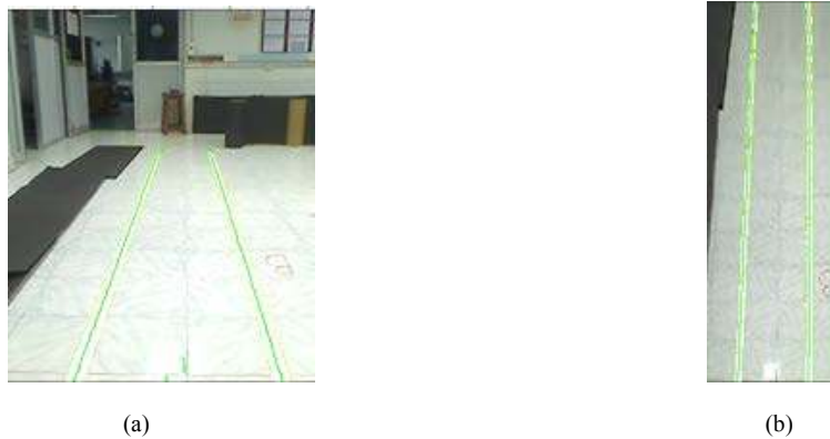
Fig. 3. Region of interest (a) Lane detected; (b) IPM of the image
