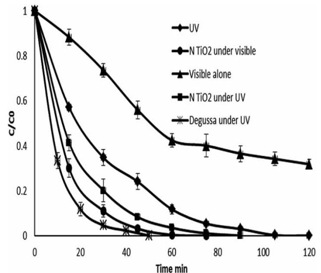
Figure 2 | Effect of photocatalyst and light source on bacterial inactivation.
