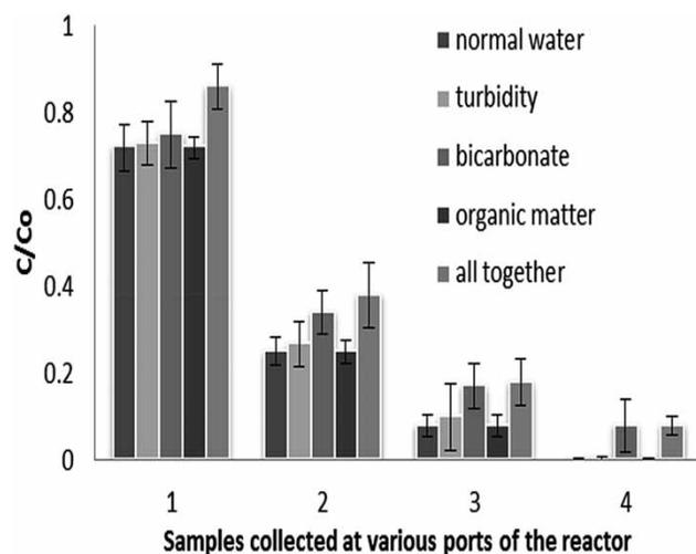
Figure 3 | Effect of inhibitory substances on survival ratio of *E. coli* during the continuous operation of the reactor (samples collected after contact time).
