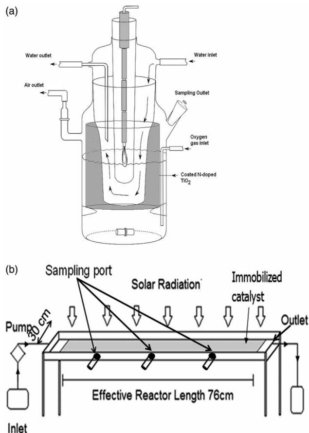
Figure 1 | Block diagrams of (a) batch reactor and (b) thin film continuous photo reactor.
