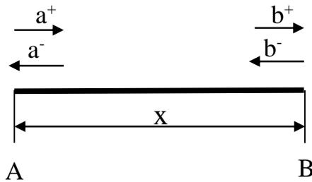
Figure 1. Waves in uniform beam.
