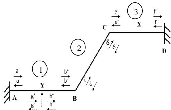
Figure 5. Waves in angular frame
