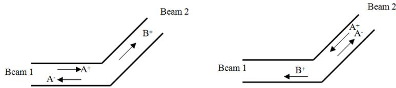
**Figure 3.** Wave reflection and transmission at an angular joint
