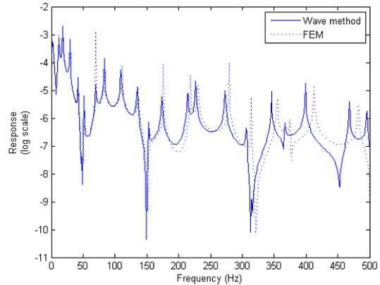
**Figure 9.** Response amplitude at x with force applied at Y for  $\Theta=35^\circ$  frame
