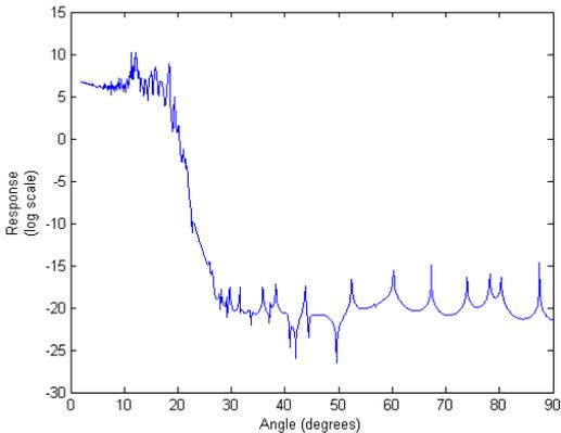
**Figure 10.** Response amplitude at x plotted as a function of  $\theta$  at frequency=2000Hz
