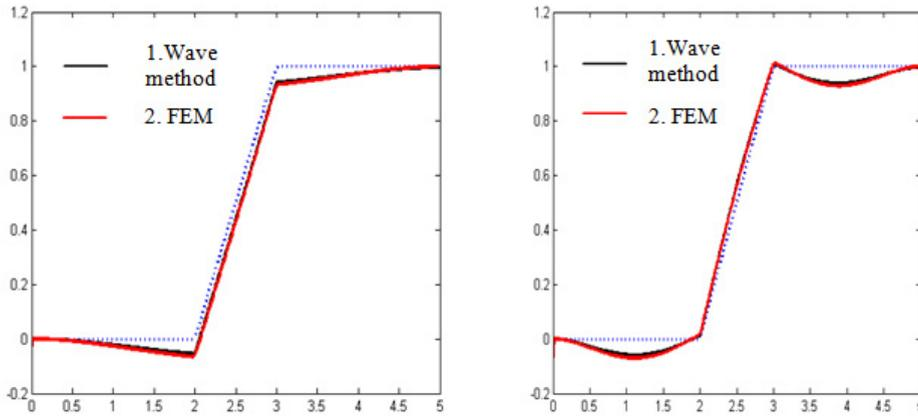
**Figure 6.** Comparison of first two modes shapes of  $\Theta=45^\circ$  frame. The unreformed shape is shown as dotted line.
