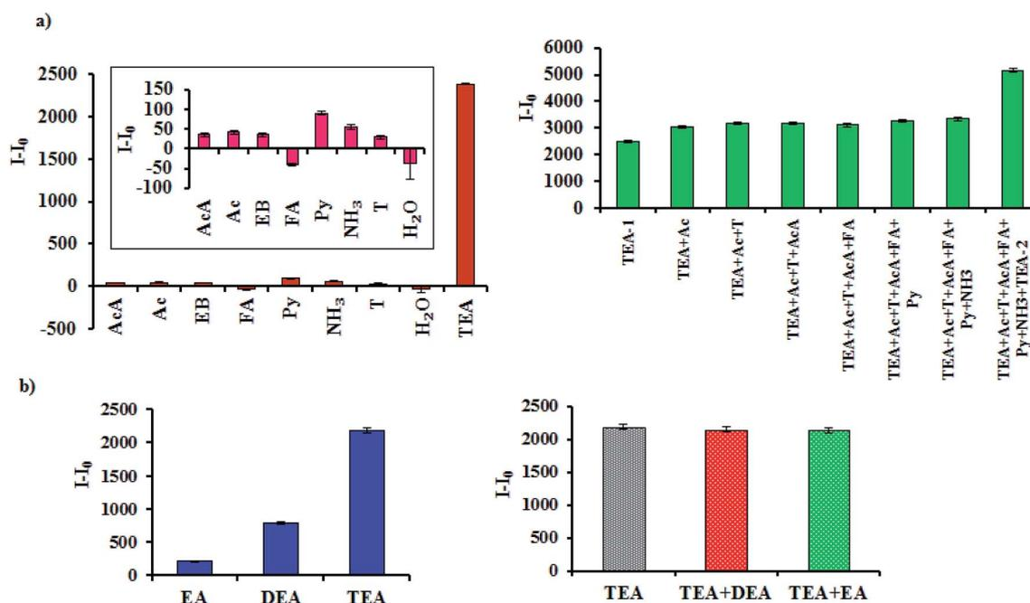
Fig. 2 The selectivity profile of Al-MOF towards TEA with common co-existing pollutants (a) and family of ethyl amines (b) (MOF and pollutant concentration:  $1\text{ g L}^{-1}$  and  $0.49\text{ mM}$ , respectively).
